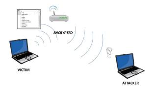
The victim is using Google search over a standard WPA/WPA2 encrypted WiFi connection. The attacker can capture the packets being transferred from victim to the access point using the monitor mode of his/her WiFi adapter. The captured packets include all types of packets going in the air. The attack is to look at the packet dump and identify what the particular user is searching.
